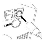
**2** Maker sure power switch is in the **0FF** position. Plug the charger into the charger port. The light on the charger should turn red during charging then back to green when charging is complete.
