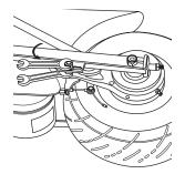
With two 8mm wrenches, loosen brake housing anchor and disconnect. Keep the spacer and washers together.
