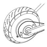
Slide rear frame cap on axle adjuster bolt.
