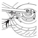
**2** If the brake lever adjuster is threaded outward and the brake still has too much slack, use the back brake adjuster at the rear brake for additional adjustment.
