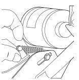
Install the brake spring and thread the cable wire into the cable anchor. Thread the cable to its original position and tighten securely.
