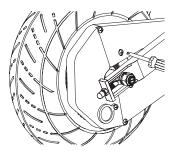
1 Loosen screws and remove chain guard.
