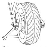
Loosen and remove both axle adjuster nuts.
