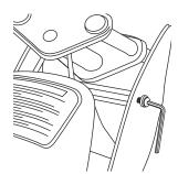
**3** If you have trouble aligning holes, put one screw in place loosely and maneuver opposite side into position. Tighten all screws.
