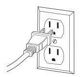
**2** Plug the charger plug into a wall outlet.
