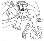
**1** Remove valve extender/adapter from right handgrip.
