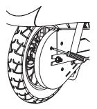
**1** With a Phillips screwdriver, remove the screws that secure the chain guard. Remove chain guard.
