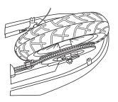
**5** Install the new chain or wheel by slipping the chain around the axle. Slide the axle into the slots on the frame. Slide the wheel forward and maneuver the chain onto the rear sprocket, motor shaft and chain tensioner.
