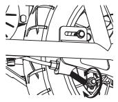
**2** If brake is too tight or has too much slack, use a 10mm wrench to loosen the nut for additional adjustment on the brake cable on the rear wheel. Securely tighten nut when done.
