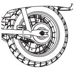
**7** Tighten the brake housing anchor securely.
