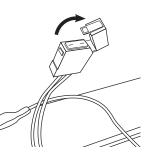
**2** Locate fuse box on top of battery. Open the fuse cover to expose the fuse.
