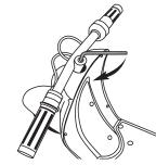
**1** Remove plastic protector and insert handlebar assembly through front fairing and into fork until it stops. Raise to desired height keeping the handlebars and fairing aligned within the red arrows of the safety zone.
