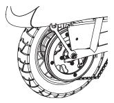
**4** With two 15mm wrenches, loosen the axle. Slide the wheel forward to loosen the chain and remove the wheel. Note the sequence of the hardware. **Note:** Your hands will get greasy doing this.
