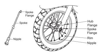
**1** Verify spoke tension by grasping and shaking each spoke. Spoke should not be loose from hub. Look for any play between spoke flanges where it mates with hub. Try to turn nipple using your fingers. You should not be able to spin any nipple by hand. If one or more spokes are loose, or if you can turn any nipple using your fingers, all spokes must be checked and need to be tightened with a spoke wrench.
