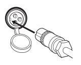
1 Turn power **OFF** before charging. Plug the charger into the charger port.
