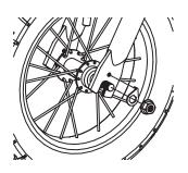
**3** Insert the tab on the lock washer into the hole on the front fork and tighten the nuts using two 15mm wrenches.
