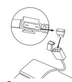
**3** Remove the fuse and replace with a new one of equal amperage. **Note:** Amperage rating is located on top of fuse.
