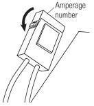
**4** Close the fuse box. Replace seat/storage compartment with the four (4) Phillips head screws.
