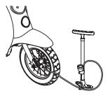
**1** Using a bicycle style tire pump equipped for a Schrader-type valve, inflate the tires to the PSI indicated on the sidewall of the tires
